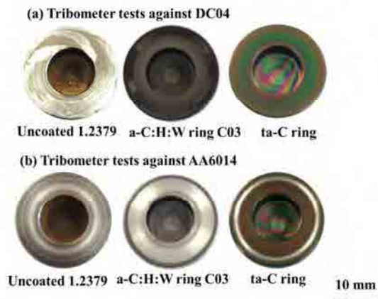
Fig. 12: The wear tracks on tested rings against (a) DC04 and (b) AA6014
