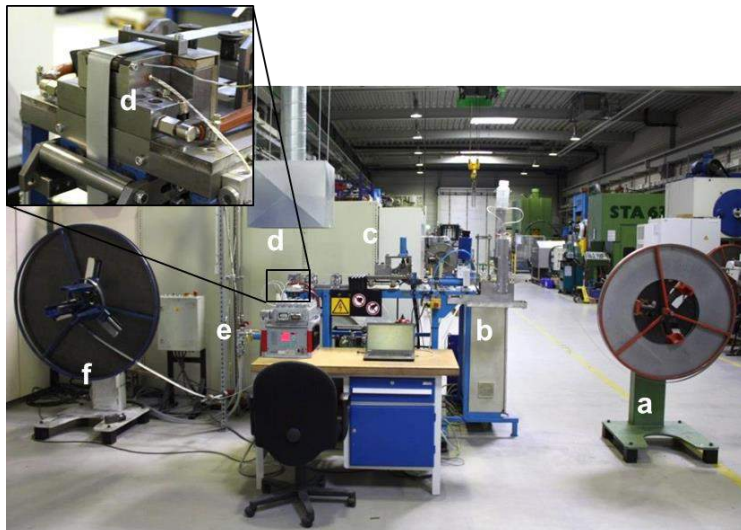
Fig. 2: left picture: Wear test bench with relevant units; a) decoiler, b) cleaning station, c) counter slide, d) specimen, e) pulling slide, f) coiler; right picture: principle of wear test bench
